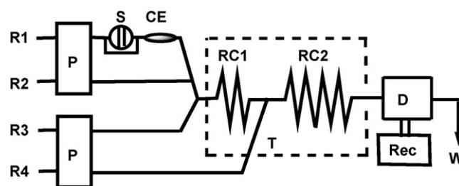
**Fig. 1.** Flow system for the determination of molybdenum(VI). R1–R4, reservoir; P, pump; S, sample injector; CE, cation exchange column; RC1 and RC2, reaction coils; T, thermostated bath; D, detector; Rec, recorder; W, waste. Conditions as in Table 2.
